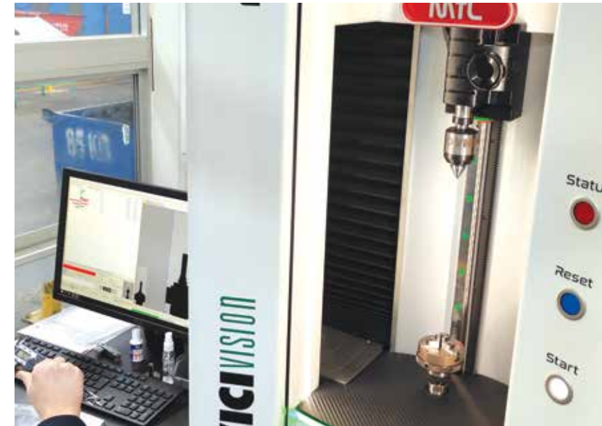
DIMENSIONAL CONTROL BY OPTICAL MEASURING DEVICE (SPC)
