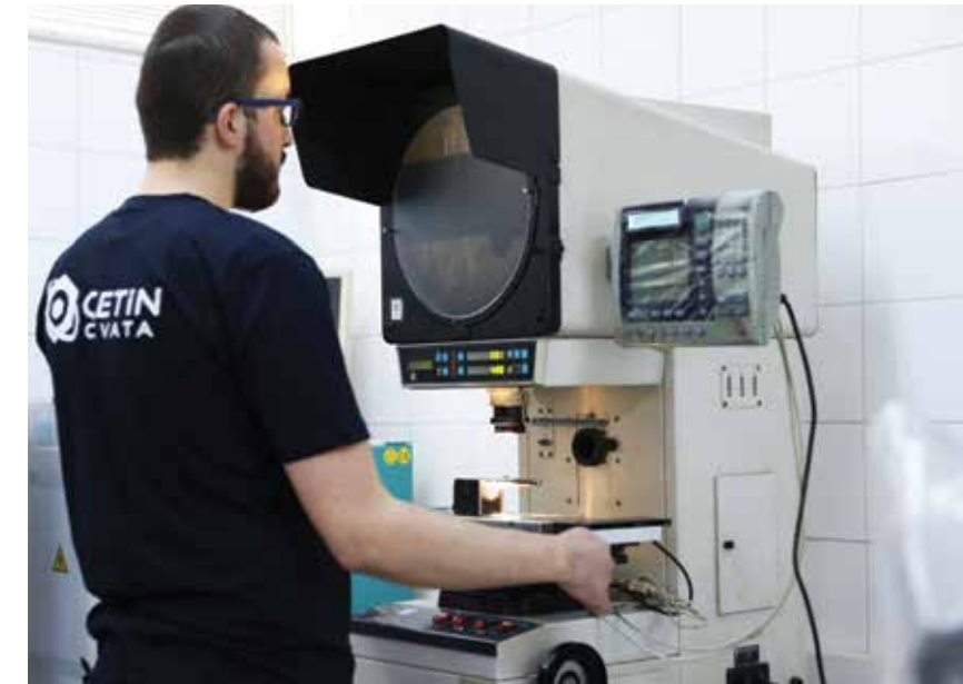
PRODUCT DETAIL CONTROL BY PROFILE PROJECTOR
