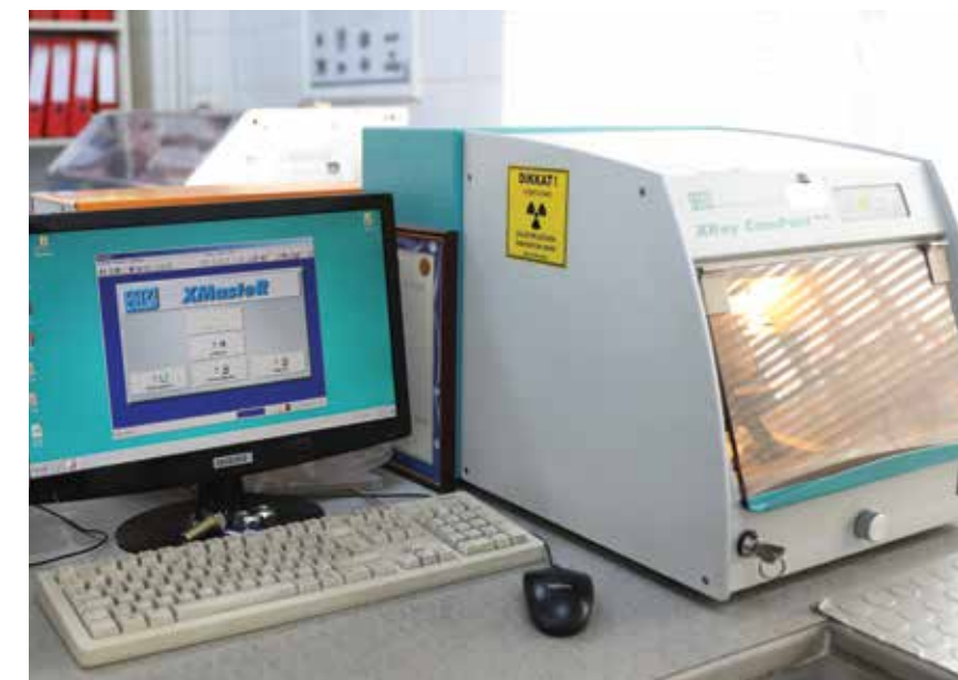
MEASUREMENT OF SURFACE COATING THICKNESS BY X-RAY DEVICE
